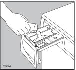
If required, pour fabric softener into the compartment marked \$\mathbb{\mathbb{G}}\$ (the amount used must not exceed the "MAX" mark in the drawer). Close the drawer gently.
